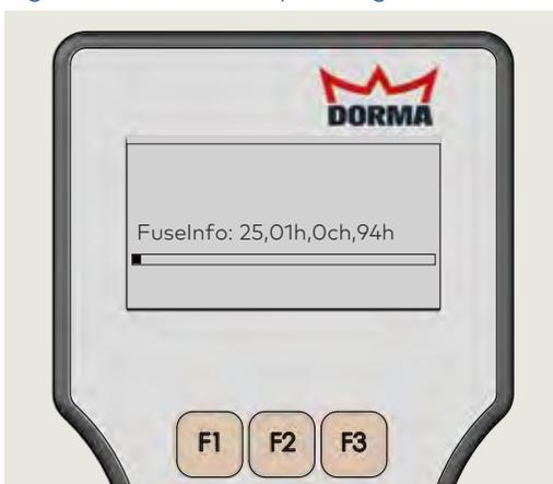
8. Firmware uploading to controller. Wait time of 3 to 5 minutes to upload.
