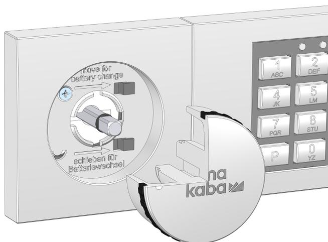
5. Mount the rotary knob on the undrilled end of the square shaft where the O-ring is attached.
