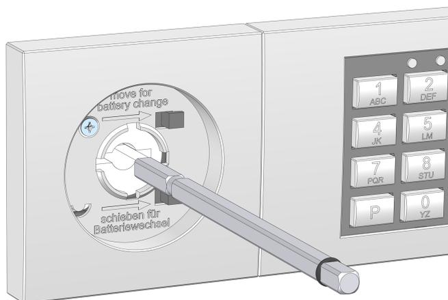
4. Insert the square shaft with the end of the bore forwards into the lock.
