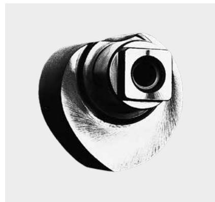
The heart-shaped cam disc and the linear drive that are a distinctive feature of all dormakaba slide channel door closers ensure easy operation of the door thanks to rapidly decreasing opening torque. This means that even children, the elderly and the disabled can open doors with ease.
