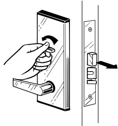
When the dead bolt is activated, keycards that cannot override a dead bolt will get a flashing yellow light and will not be able to open the door. The Security/Emergency key and any guest keys that are programmed to override a dead bolt will get the normal flashing green light instead and will be able to open the door.
