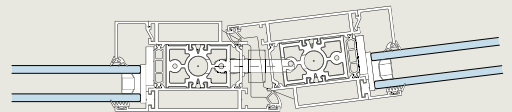
Standard profile interlock with double-offset sealing arrangement implementable up to an angle of 7°
