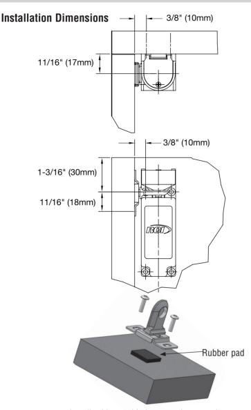
Install rubber pad in between the mounting surface and catch to secure catch position
