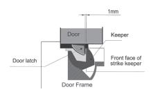
As drawn in the diagram, there should be a 1mm gap between the door latch and the front face of the strike keeper, preventing the door from creating back pressure on the strike keeper when the door is closed. This gap is important to ensure the proper functioning of the strike.
