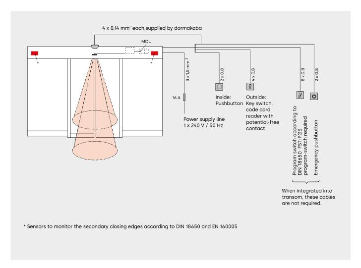
The external emergency pushbutton has to be installed in the close range of the door. Max. cable length: 50 m. Can be run in one cable with the program switch.
