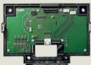
Docking station for PoE data line with "option door control"
