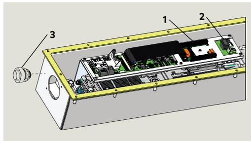
Fig. 16.8.2 115 Vac terminal block
