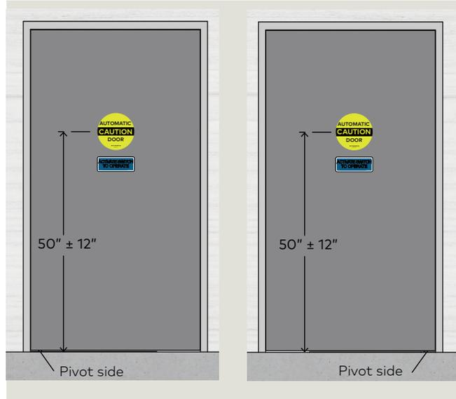
Fig. 12.3.2 Push/Pull Push To Operate
