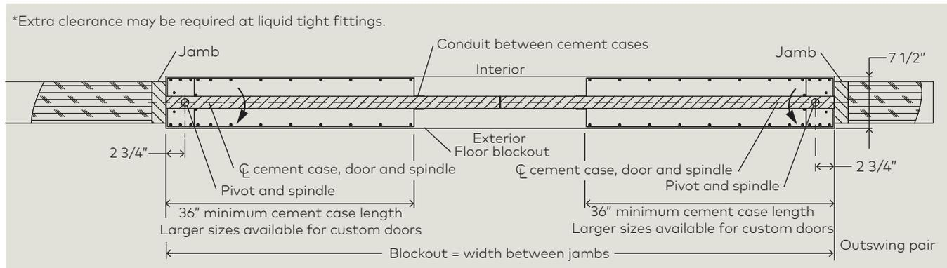
Fig. 13.1.5 Double door center hung front view
