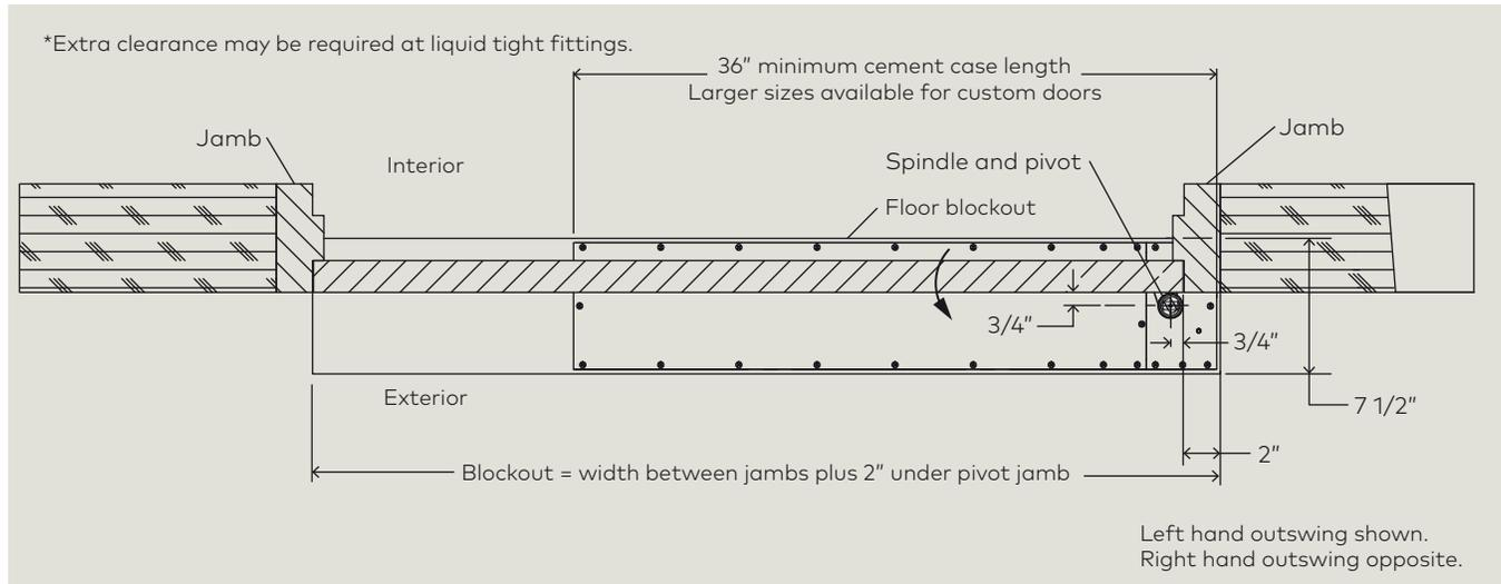
Fig. 13.2.3 Single 3/4" offset pivot door front view
