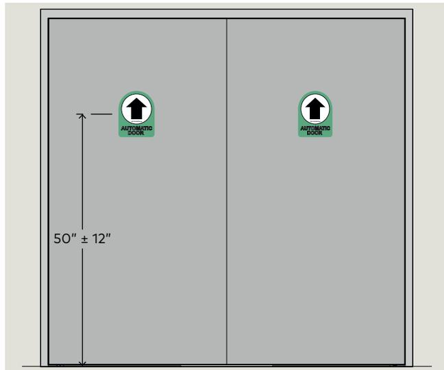
Fig. 12.5.2 One way traffic, non approach side
