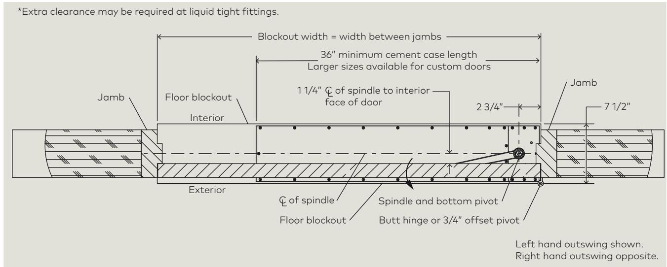
Fig. 13.3.3 Arm and track single door front view
