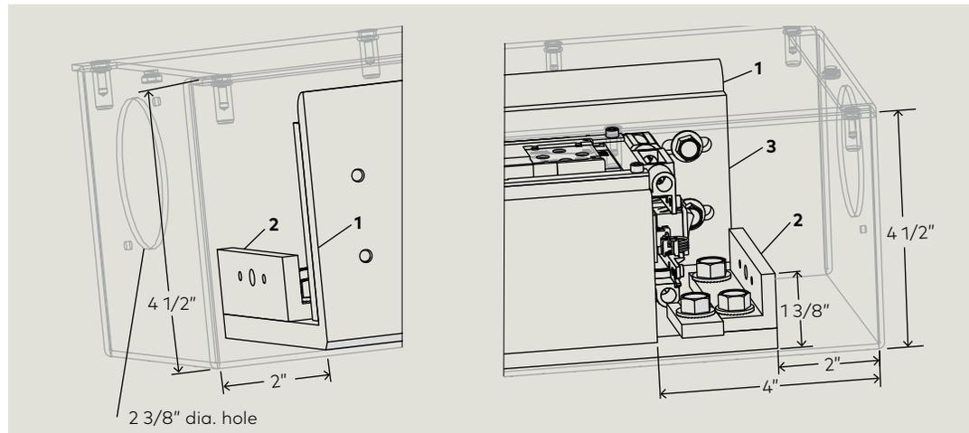
Fig. 15.5.2 Cement case end (opposite spindle side) areas for conduit entry
