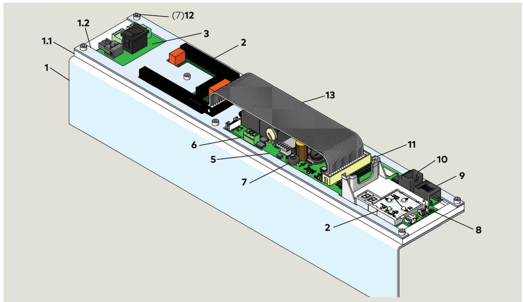
Fig. 6.2.4 Operator communication connectors, upgrade card slot
