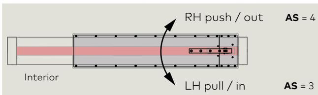
Fig. 16.15.2.6 Center hung arm, pivot at left jamb
