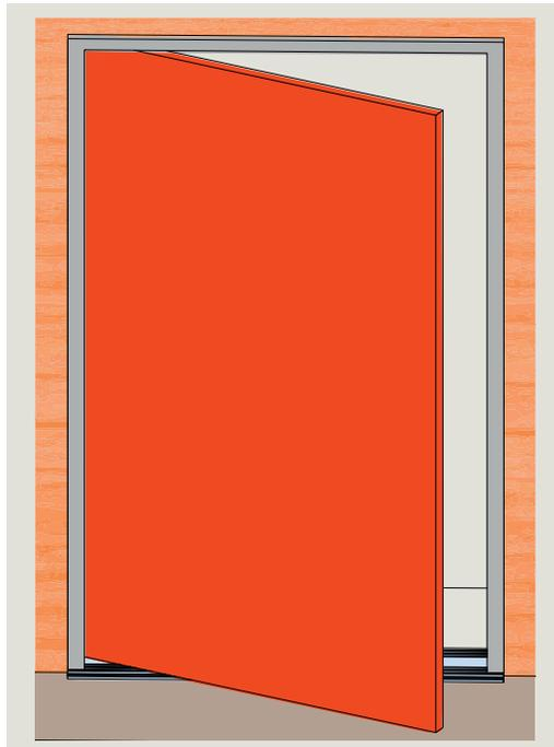
Fig. 4.2.2.1 Center hung arm and top pivot
