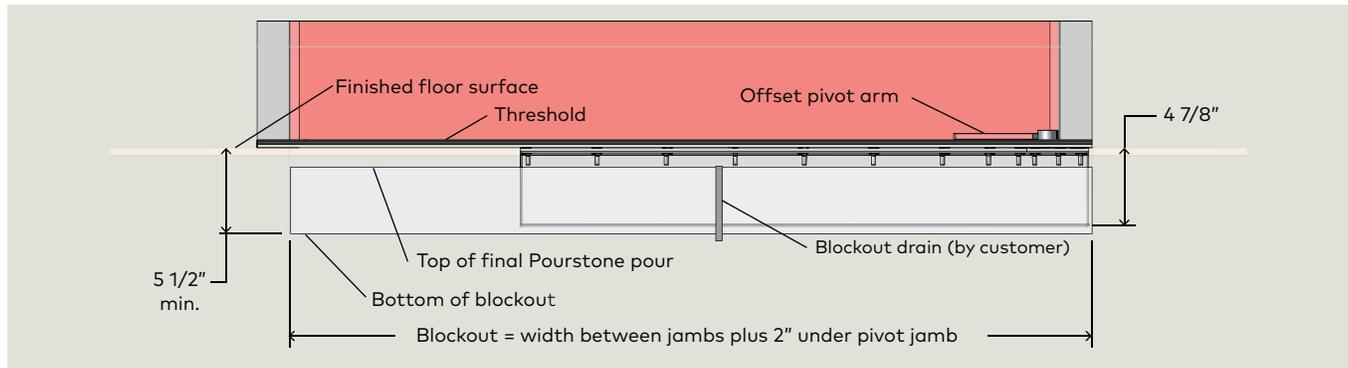
Fig. 13.2.4 Double door 3/4" offset pivot
