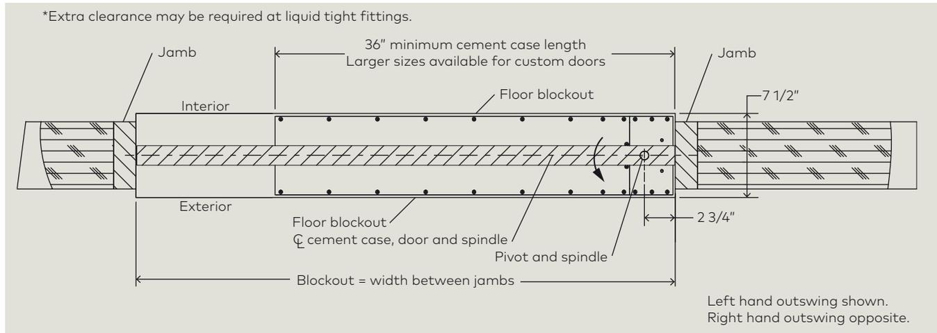
Fig. 13.1.3 Single door center hung front view
