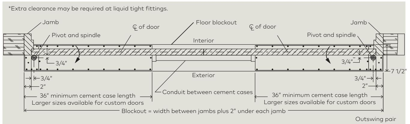
Fig. 13.2.5 Double door 3/4" offset pivot front view
