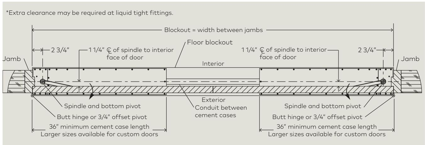
Fig. 13.3.5 Arm and track double door front view
