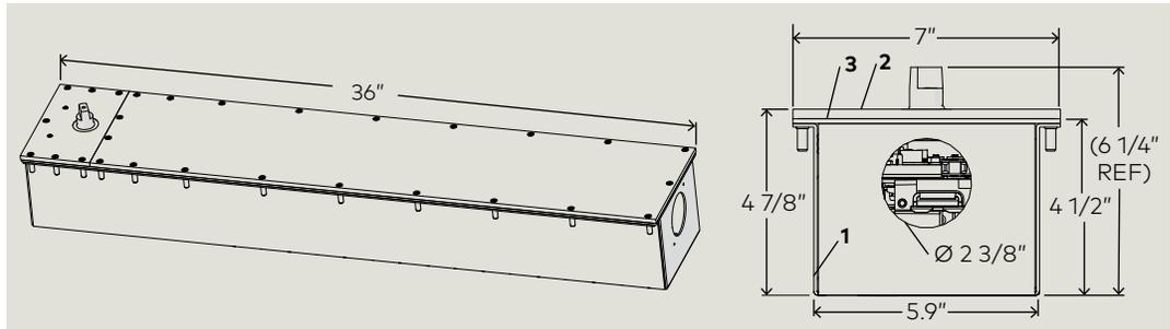
Fig. 6.1.2 ED250 in-ground case cover and fasteners
