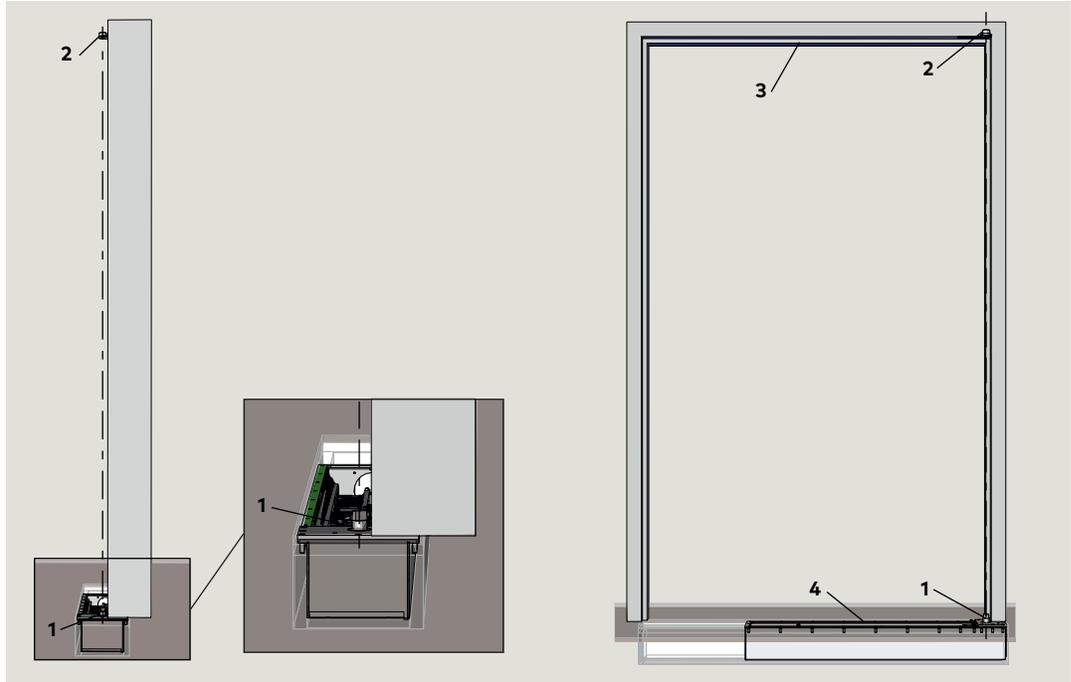
Fig. 16.4.2 LH center hung door, alignment of spindle with top pivot
