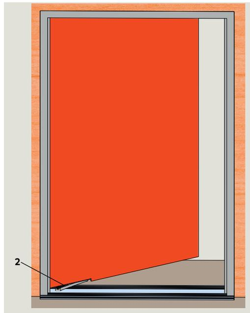
Fig. 4.3.1.1 Arm with track, butt hinge
