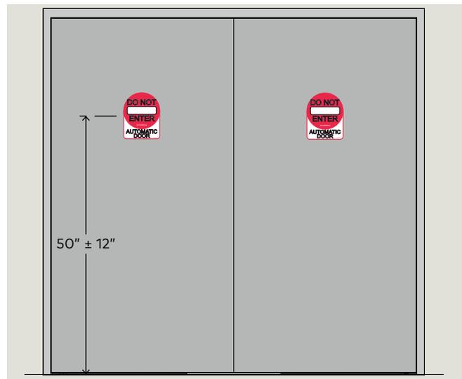
Fig. 12.5.3 Two way traffic, non swing side
