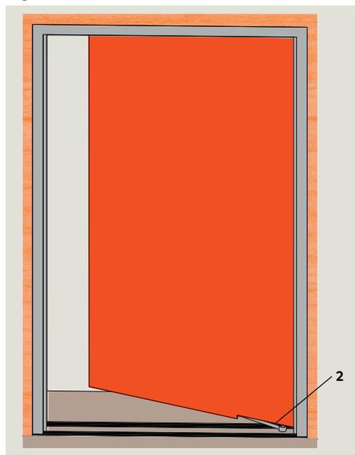
Fig. 4.3.2.1 Arm with track, butt hinge
