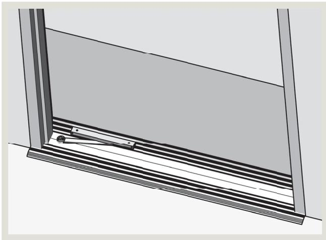
Fig. 28.1.3 Threshold installation end view example
