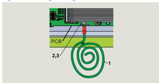
Fig. 15.2.3 ED250 case with ground lug installed
