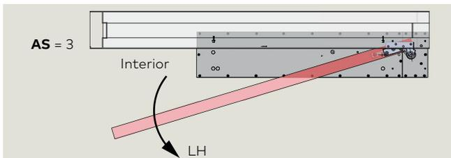
Fig. 16.15.2.5 Center hung arm, pivot at right jamb
