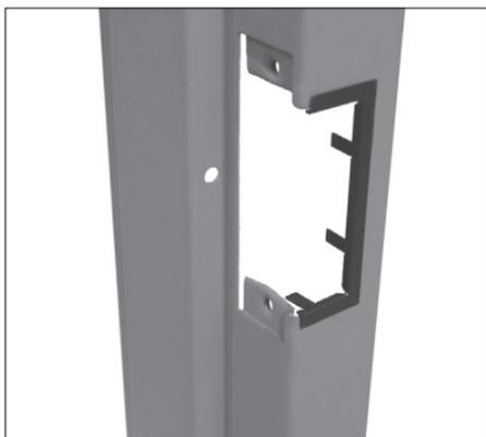
Make sure the Trim Plate series label matches the Strike series you are installing.
