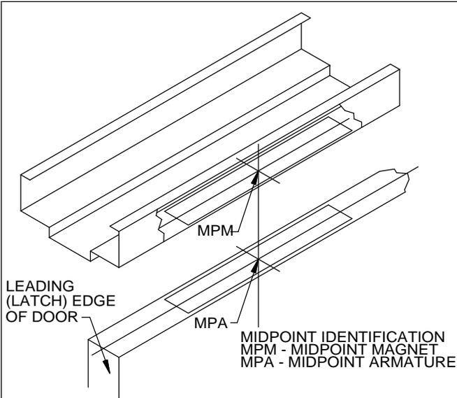
THE MOST IMPORTANT ELEMENTS FOR THE PROPER INSTALLATION OF THE EMSL-2000 MAGNET ASSEMBLY ARE THAT THE MIDPOINT OF THE ARMATURE, AND THE MIDPOINT OF THE MAGNET MUST LINE UP EXACTLY. ALL CENTER LINES OF THE ARMATURE MUST LINE UP WITH THE RESPECTIVE CENTER LINES OF THE MAGNET.
