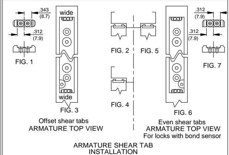
Please note drawing FIG. 1. shows two different alignments off center of the shear tab.
