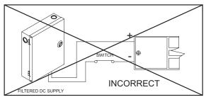
Fig. 2 – Power Connections
