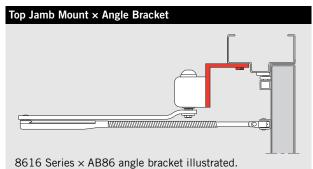
To provide clearance for surface applied stop/holder. See table above for other closers.
