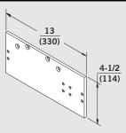
DP86FC — For top jamb mount with full plastic cover to clear a surface applied stop/holder. Overhead ceiling clearance must be 1-3/4" (44 mm) or more. Permits parallel arm installation with minimum top door rail of 2-1/2" (64 mm) for non-hold open, 2-3/4" (70 mm) for friction hold open applications (assuming 5/8" [16 mm] stop dimension).
