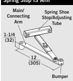
Provides a spring assisted dead stop function for regular and top jamb applications at 85°, 90°, 100°, and 110°. Arm is non-handed.
