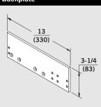
**BP86TFC** — For use with pull-side track applications with full cover (closer on frame face, track on door) to permit installation on a standard 2" (51 mm) frame face.
