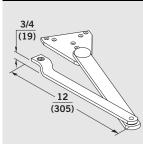
Heavy-duty parallel arm. Available in non-hold open and thumb turn hold open. Units can be installed for maximum opening of 100° or 180°. Hold open units will hold open at 90° or 125°. Maximum opening is 180° (conditions permitting). Arm is non-handed. Non-hold open arm illustrated.
