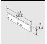
**BP74T** — For use with pullside track applications (closer on frame face, track on door) to permit installation on a standard 2" (51 mm) frame face.
