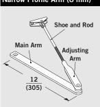
**ARNP** — Complete arm assembly. Regular or top jamb mount. Permits installation on 1" (25 mm) frame face for regular mount with maximum pull-side reveal of 1/8" (3 mm). Can also be used top jamb (0"-4" [0 mm-102 mm] reveal) for narrow top door rails. Arm is non-handed. **ARNPP** — Complete arm assembly for parallel arm mount (Tri-Pack). (0"-4" [0 mm-102 mm] reveal). P86 included.
