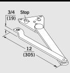
Heavy-duty parallel arm with integral cushioned opening function. Available in non-hold open, thumb turn hold open, and hex key turn hold open. Units can be installed to achieve either stop or stop and hold open at 85°, 90°, 100°, and 110°. Maximum opening is 110° (conditions permitting). Arm is non-handed. Nonhold open arm illustrated.
