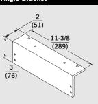
AB74 — For installation of closers where parallel arm and top jamb applications are not practical due to low overhead ceiling clearance, narrow frame face or unusual trim conditions. This bracket can also be used to provide clearance for a surfaceapplied stop/holder.
