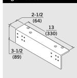
AB86 — For installation of closers using a slim or full plastic cover. Used where parallel arm and top jamb applications are not practical due to low overhead ceiling clearance, narrow frame face or unusual trim conditions. This bracket can also be used to provide clearance for a surface-applied stop/holder.
