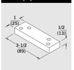
**BS** — For use with all 7400 Series P86, PD, and PHB applications installed on cased frames with applied blade stops. This block is used to provide adequate clearance for the blade stop.
