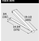
Provides slide track function for improved aesthetics and vandal resistance. Units can be installed to provide 85°,  $90^{\circ}$ ,  $110^{\circ}$ , or  $180^{\circ}$  of door opening (conditions and application permitting). Arm is non-handed.
