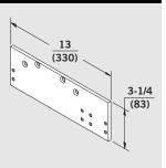
**BP86FTFC** — Required for track mount with full cover when being used on a flush transom (closer on transom, track on door). Mounting holes in the plate avoid rabbet on door.
