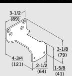
**PFT** — For all 7400 Series closer hold open and non-hold open parallel arm applications where flush transom conditions prohibit use of P86 or PHB bracket.
