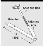
**ARNPJ** — Complete arm assembly for top jamb installations (4"-8" [102 mm-203 mm] reveal) for narrow top door rails. Arm is non-handed. AMR48NP — Narrow profile main arm and adjusting arm. Used in conjunction with SR48 shoe and rod. Uses 10 mm rod.
