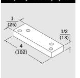
**BSHD** — For use with all 7400 Series DS and SPA applications installed on cased frames with applied blade stops. This block is used in conjunction with the spacer furnished with the arm to provide adequate clearance for the blade stop.
