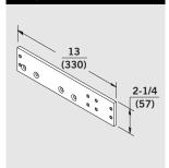
**BP86T** — For use with pullside track applications (closer on frame face, track on door) with slim plastic cover to permit installation on a standard 2" (51 mm) frame face.
