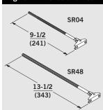
SR04 (8 mm Rod Diameter) — 0"-4" (0 mm-102 mm) reveal. Shoe and rod only. SR48 (10 mm Rod Diameter)— 4"-8" (102 mm-203 mm) reveal. Shoe and rod only. SR04 has an 8 mm rod and must be used in conjunction with main arm and adjusting arm AMR04. The SR48 has a 10 mm rod and must be used with main arm and adjusting arm AMR48. Non-handed.
