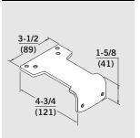
**PHB** — Furnished standard with 7400 Series friction hold open parallel arm applications.
