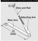
ARJ — Complete Arm Assembly (4"-8" [102 mm-203 mm] reveal) with 10 mm rod. Designed specifically for top jamb applications with deeper reveals. Arm is non-handed. AMR48 — Regular non-hold open main arm and adjusting arm. Accepts 10 mm rod.
