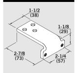
MJ — For 7400 Series closers with regular mount non-hold open assemblies, where frame conditions will not permit use of the standard foot, e.g. molded or ornate trim. Permits use of parallel arm application between twin communicating doors where limited space prohibits use of the wider P86 bracket.
