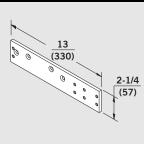
**BP86** — For top jamb mount with slim plastic cover when overhead ceiling clearance is less than 2-1/4" (57 mm). Can also be used for regular mount to clear a mortised overhead stop/holder.
