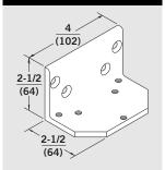
**FTHD** — For use with all DS and SPA applications where flush transom conditions prohibit normal installation of soffit bracket.
