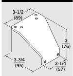
**PD** — For 7400 Series closer non-hold open parallel arm applications to clear a surface-applied stop/holder.
