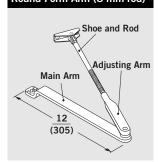
AR — Complete Arm Assembly (0"-4" [0 mm-102 mm] reveal) with 8 mm rod. Arm is non-handed.
