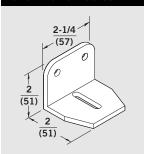
**NFHD** — For use with all DS and SPA applications where total frame depth is less than 4-1/2" (114 mm), prohibiting use of standard spacer block. NFHD bracket is used in lieu of block supplied with arm.
