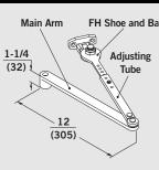
Provides a hold open function between approximately 90° and 180° of door opening (conditions permitting). Arm is non-handed.
