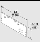
DP86 — For top jamb mount with slim plastic cover to clear a surface applied stop/holder. Overhead ceiling clearance must be 1-3/4" (44 mm) or more. Permits parallel arm installation with minimum top door rail of 2-1/2" (64 mm) for non-hold open, 2-3/4" (70 mm) for friction hold open applications (assuming 5/8" [16 mm] stop dimension).
