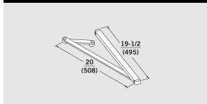
Provides slide track function for pull-side reveal conditions up to 3-1/2". Provides 117° of door opening (conditions permitting). Arm is handed. Also available with hold open option to provide selective single point hold open between 30° and 110°.
