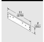
**BP74** — For top jamb mount when overhead ceiling clearance is less than 2-1/4" (57 mm). Can also be used for regular mount to clear a mortised overhead stop/holder.
