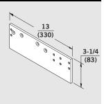
BP86FC — For top jamb mount with full plastic cover when overhead ceiling clearance is less than 2-1/4" (57 mm). Can also be used for regular mount to clear a mortised overhead stop/holder.
