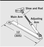
AO8 —Complete secured elbow arm non-hold open assembly (0"-4" [0 mm-102 mm] reveal) with 8 mm rod. Optional arm with 7400 Series closers. Arm is nonhanded.
