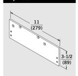
DP74 — For top jamb mount to clear a surface applied stop/holder. Overhead ceiling clearance must be 1-3/4" (44 mm) or more. Permits parallel arm installation with minimum top door rail of 2-1/2" (64 mm) for non-hold open, 2-3/4" (70 mm) for friction hold open applications (assuming 5/8" [16 mm] stop dimension).
